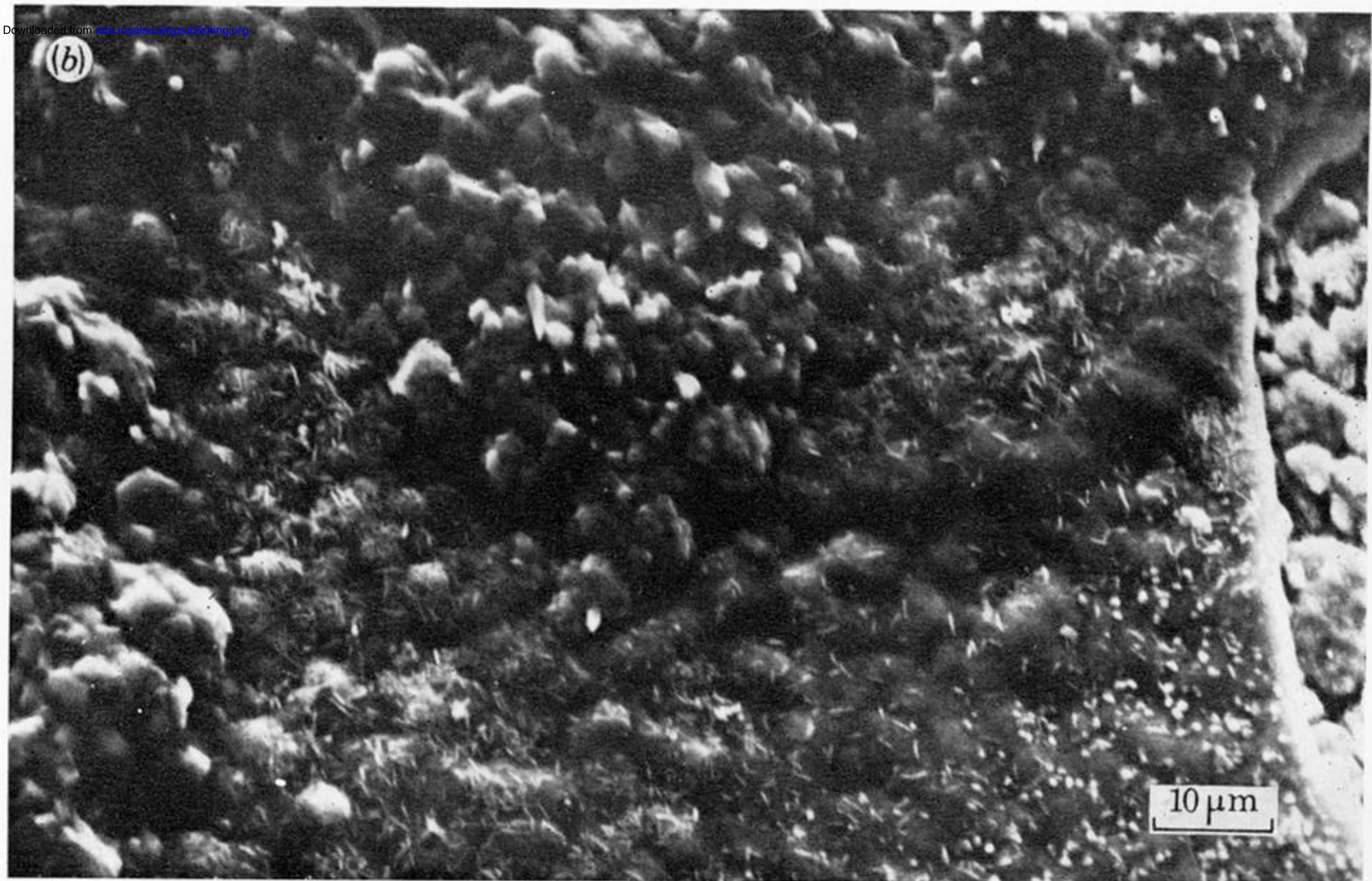
FIGURE 6 ( a, b ). The surface of the scale on sample 5. Whiskers are evident in figure 6 a but not in such profusion as on some other samples. Figure 6 b shows two regions. The scale at the top of the photograph has the appearance of an excrescence with coarse crystalline texture. The scale in the lower part of the picture is similar to that on samples oxidized for shorter times. Electron acceleration energy = 30 keV.
