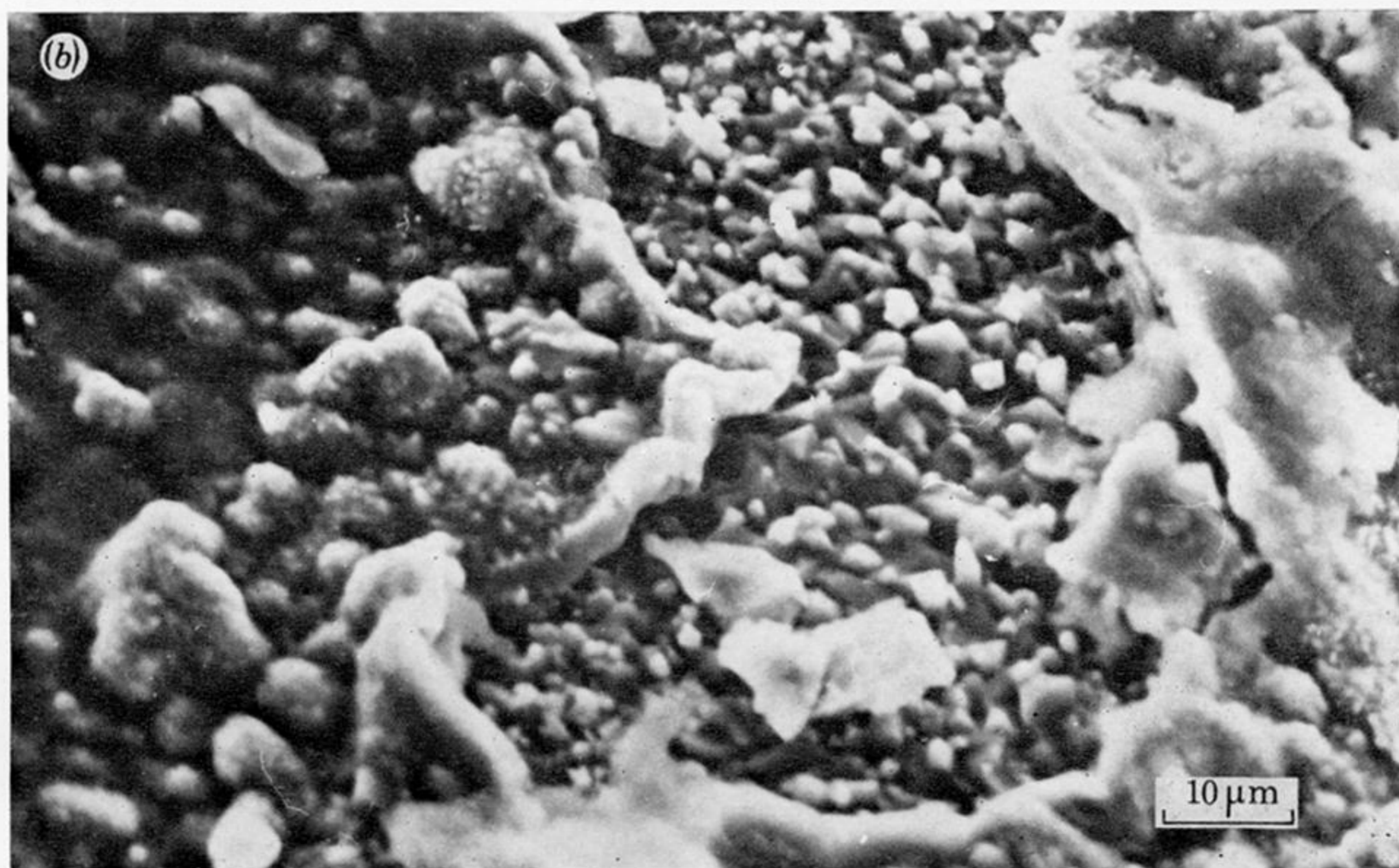
FIGURE 5 ( a, b ). The surface of the scale on sample 1. Note the broken part of the scale at the left of figure 5 a which shows that the buckled regions are areas where the scale has lifted from the alloy. Figure 5 b also shows that the scale has buckled and lifted from the surface. Electron acceleration energy = 30 keV.
